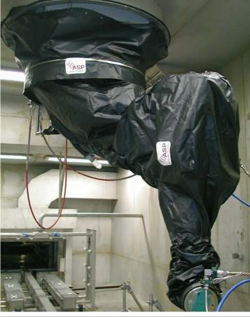
Sealed cover with welded seams
