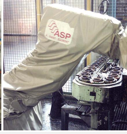
A simple, reliable solution Stands up well to lubricants Seams protected if necessary
